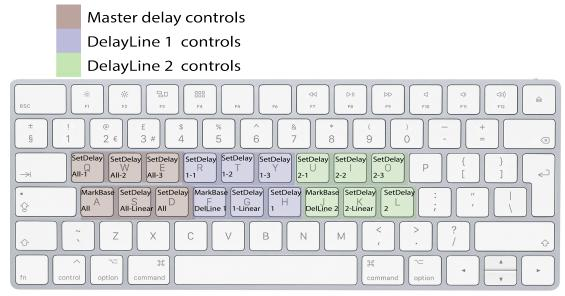
Below diagram shows the shift key layout for delay control:
